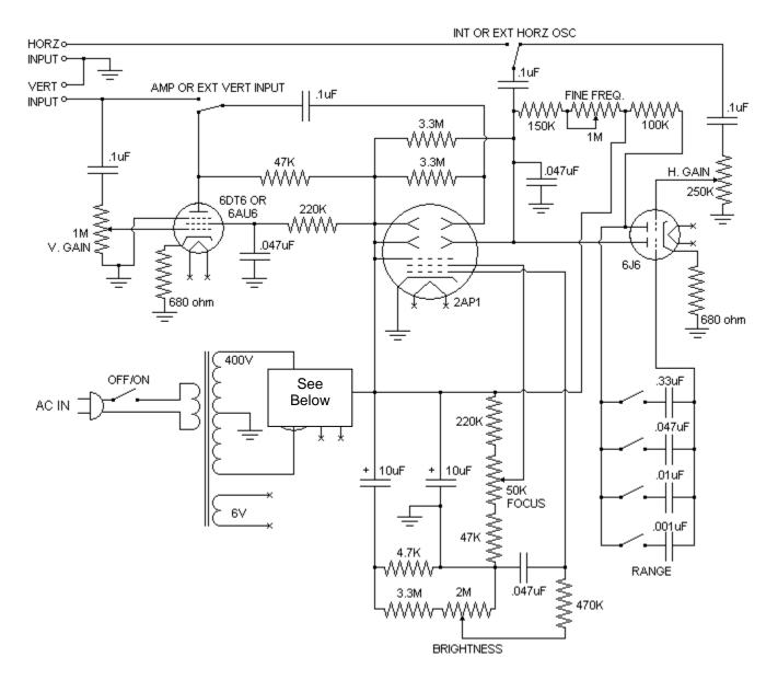
There is a flaw in the power supply in the original schematic. The 5Y3's filaments have high B+ voltage, therefore the other tubes' filaments are supplied with that B+ voltage. Those tubes have very low filament to cathode voltage ratings. This will reduce tube life or short them. It is better to provide a separate filament supply for the 5Y3 or modify the power supply for a different tube. Below is a schematic for an acceptable power supply.
